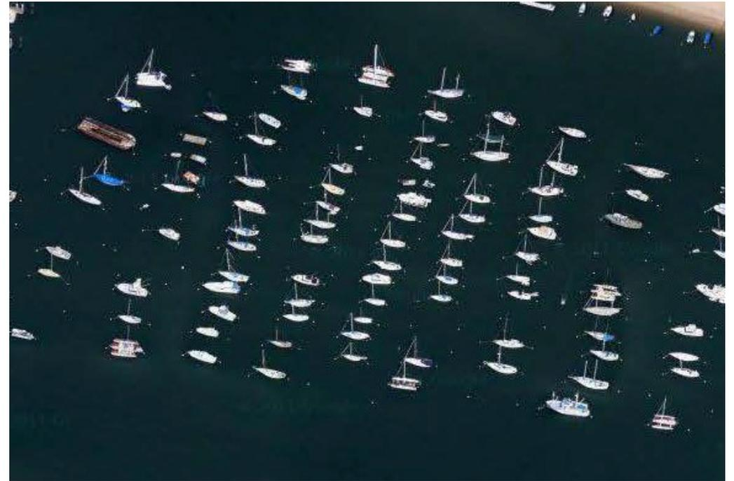
The typical 2-point mooring field above maintains consistent boat lengths in each row and clearly defined fairways for navigation. Newport Harbor mooring fields do not maintain consistency of boat lengths in rows or widths in fairways.
