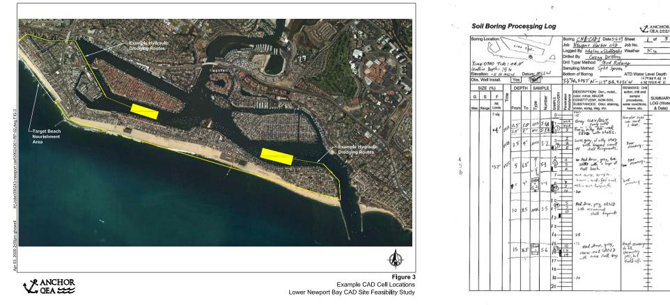
"Visual inspection of cores in the field indicated the material within the upper 5 feet of the surface typically a gray, very soft, silty clayey material that appears to be relatively recent sediment deposits. At depths below 5 feet, dense to very dense sand was encountered to the bottom of each boring." Preliminarily, this material appears to be suitable for a helical type anchor system
