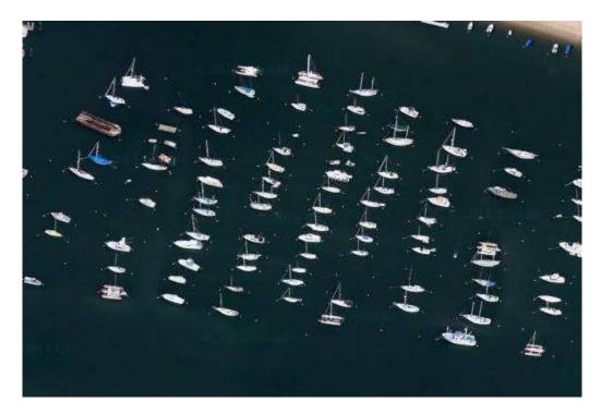
The typical 2-point mooring field above maintains consistent boat lengths in each row and clearly defined fairways for navigation. Newport Harbor mooring fields do not maintain consistency of boat lengths in rows or widths in fairways.
