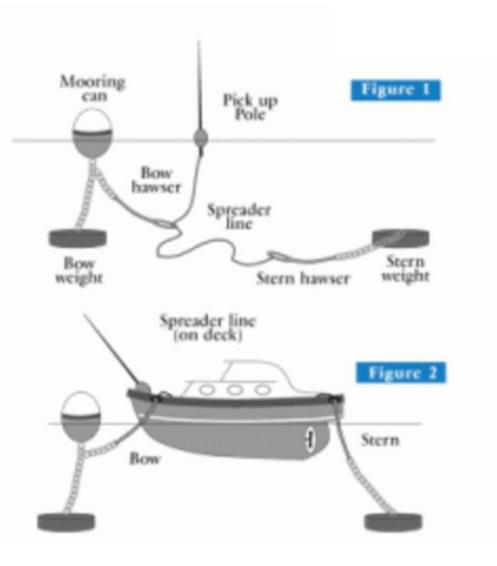
Spreader line moorings do not require the placement of a second buoy. This reduces the footprint of the mooring to a single point allowing for wider fairways between rows.
