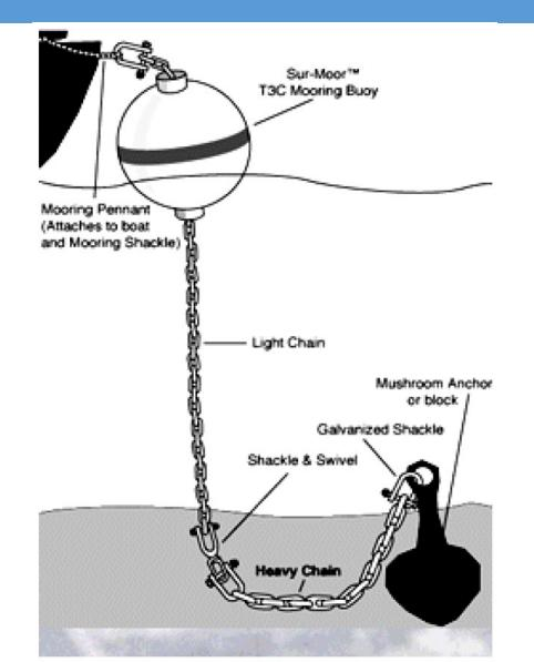
The diagram shows the typical configuration of an offshore mooring in Newport Harbor. A single two-point mooring will typically use two of the mooring configurations shown. One for the bow of the boat and one for the stern.
