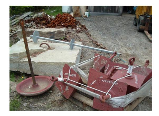
Mushroom anchor, granite block, helical, pyramid and manta (not shown).
