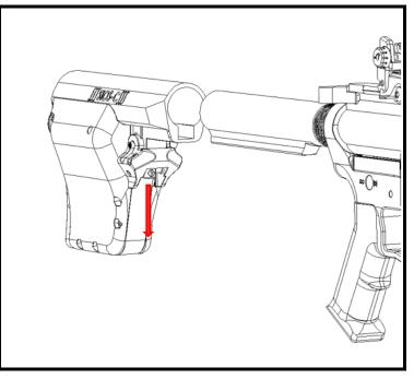
Figure 2.0.3: Installation Step Three
