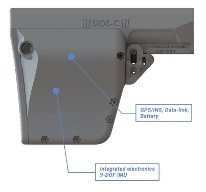
The VKIS SIOS-C11B models serve as a drop-in MIL-SPEC replacement buttstock for rifles using an AR-15 type MIL-SPEC sized receiver extension tube. The 9-DOF IMU and GPS inside the stock communicate to an Android device, passing location, orientation, and status to everyone in the group.
