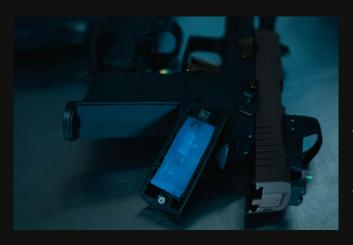
Electronics include a 9-DOF IMU (Accelerometer + Gyro + Digital Compass), Microphone, and Bluetooth. VICE-VK320 sends weapon orientation (roll + pitch + yaw) to a connected TAK device. VICE for VK320 is compatible with the SmarTak® inForce ATAK Plug-in.
