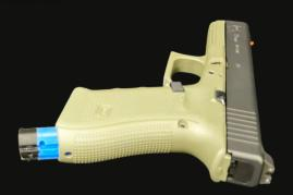
Electronics include a 9-DOF IMU (Accelerometer + Gyro + Digital Compass), Microphone, and Bluetooth. VICE for GLOCK® sends weapon orientation (roll + pitch + yaw) to a connected TAK device. VICE for VK320 is compatible with the SmarTak® inForce ATAK Plug-in.
