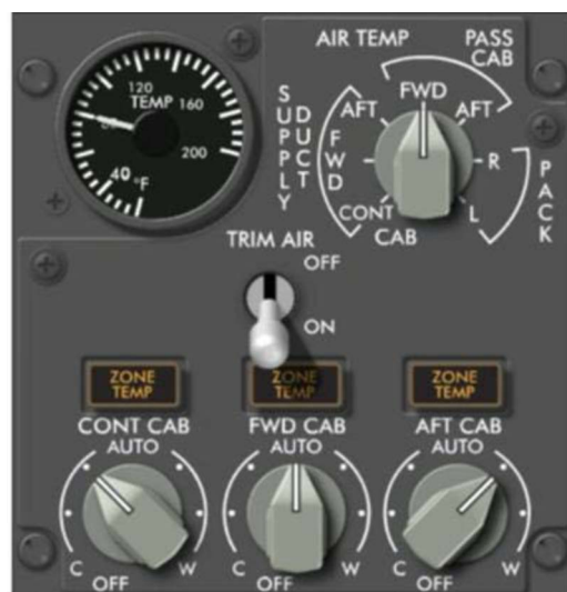
FIGURE 2-5 Representative flight-deck interfaces from Boeing 737 aircraft showing flight crew controls for cabin and flight-deck temperature setpoints used to manage thermal comfort.
