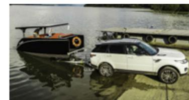
The size of the catamaran allow to transport of the boat efficiently. It can be towed by a vehicle with towing capacity of as little as 2500 pounds.
