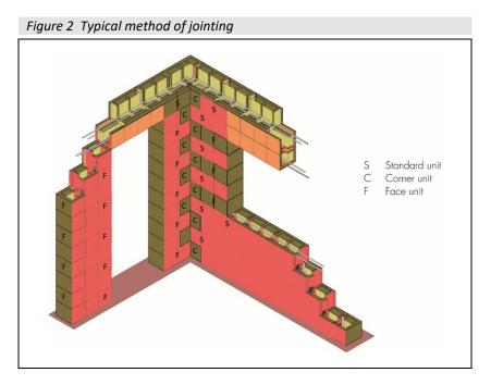
1.7 Structures with non-modular dimensions can be accommodated using standard or face units cut to suit.
