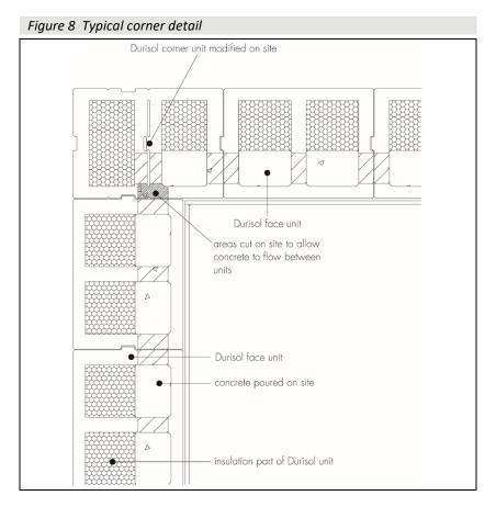
16.3 Following completion of the first course, the formwork is checked for plumb and level and the next five courses laid in a running bond. Separating or internal walls are jointed as shown in Figure 9.
