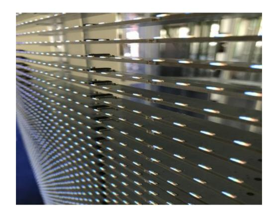
LED lamps (Customized Nation Star SMD 3806) and driver ICs are mounted on the side of the PCB, enhancing transparent rate to the maximum while reducing interferer of the view to the minimum.
