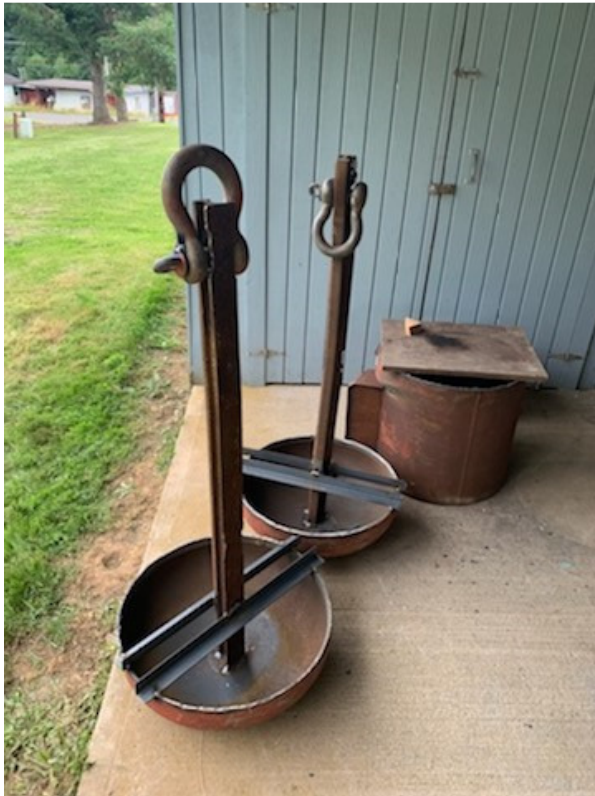
Two Heavy duty mooring anchors
