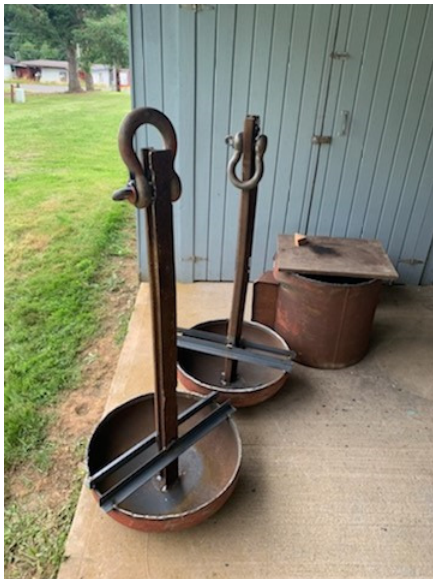
Two heavy duty mooring anchors
