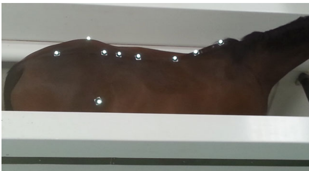
Fig 1: Horse in water treadmill showing the marker set used to measure thoracolumbar FE ROM and pelvic vertical displacement.
