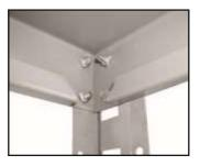
Top and bottom shelves are triple flanged at all four sides and bolted to angle posts at all four corners for maximum rigidity, durability and stability.
