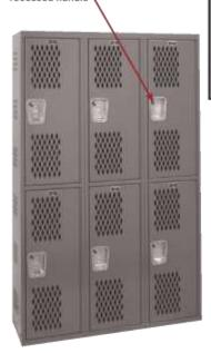
Lockers include a 3\* wide 18 gauge full height door stiffener spot welded to the inner door face and MIG welded to the hinge side as well as to the top and bottom door flanges providing a rigid torque-free door.
