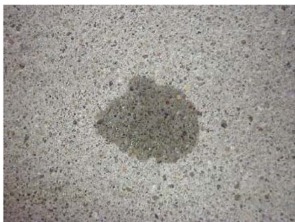
FIG. 3 Absorptive Concrete Surface
