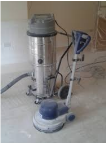
Floor sanding machine w/ shroud + dust control
