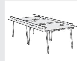
Lay the slab on a flat surface and preferably on a workbench with aluminum profiles. Make sure the surface is stable for both cutting and drilling.
