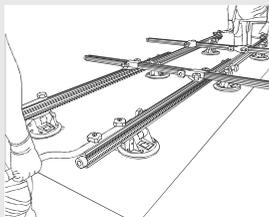
To lift the slabs use sucker cups after cleaning the slab and cups with a damp sponge. Make sure the device also has suckers that run along with the guides and adhere to the slab.
