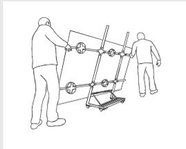
We recommend carrying out the handling job of the slabs with four handlers at the same time.
