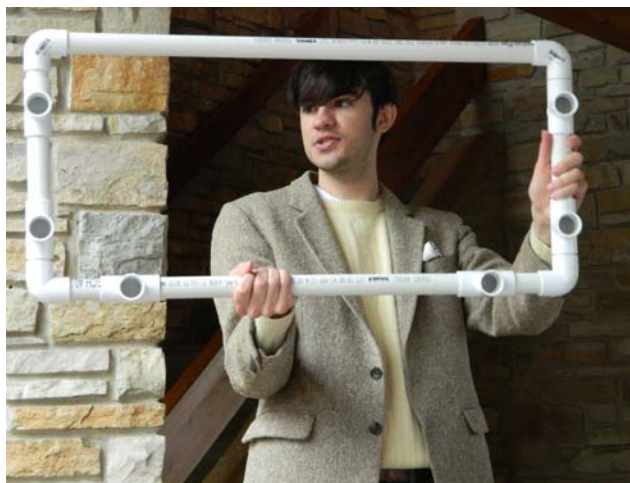
Alfonso is holding a base. Two are needed, one to support the top and one on the bottom
