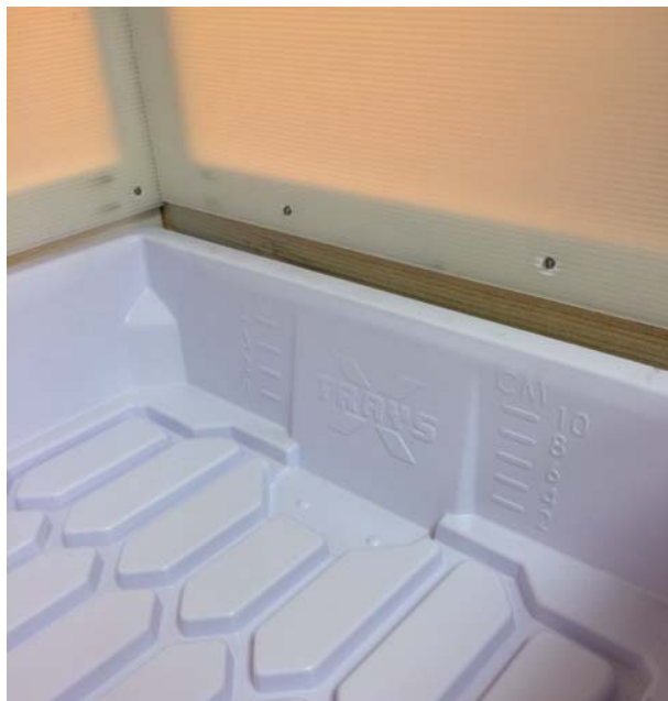
Close up of the hydroponics tray used to make the bottom water proof and sturdy with polycarbonate walls screwed in the cabinet corner supports.
