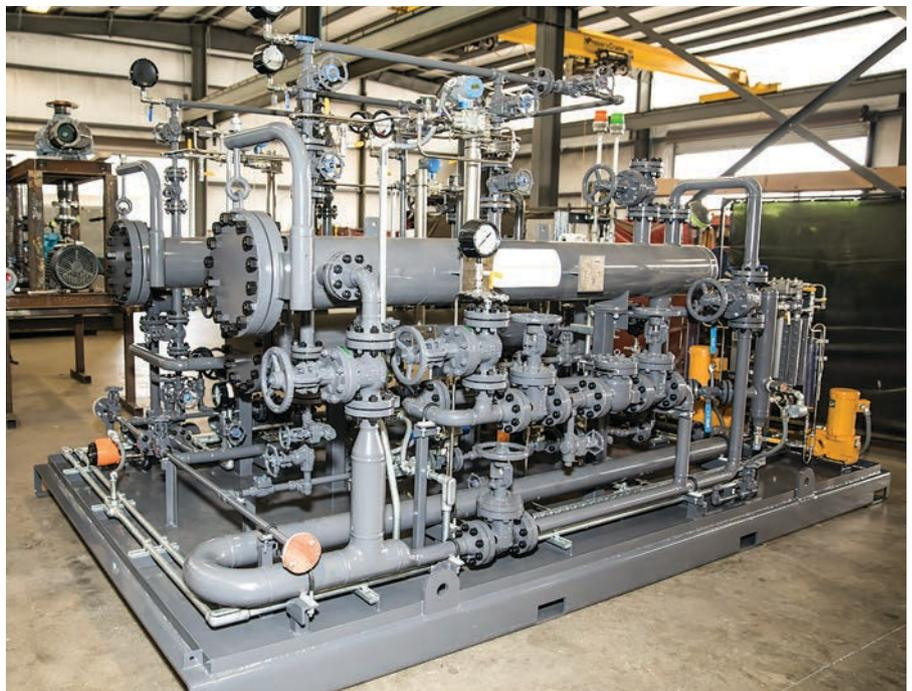
**FIG. 7.** Full-scale system<sup>b</sup> for butane treating.
