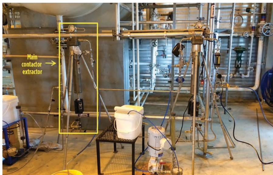
FIG. 3. Miniaturized system<sup>b</sup> used for mercaptans removal validation.
