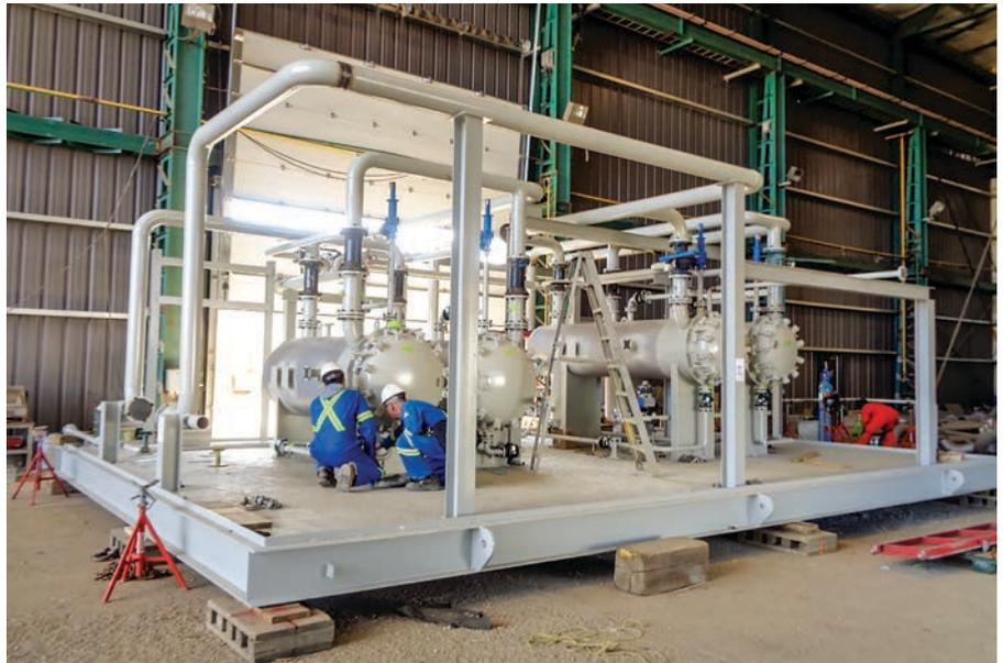
**FIG. 6.** Full-scale system<sup>b</sup> for condensate treating.
