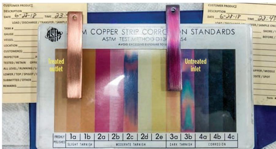
**FIG. 8.** Copper strip test results when using the system<sup>b</sup> for butane treating. The untreated copper strip test (3b result) is shown at right, and the treated copper strip test result (1b) is shown at left.
