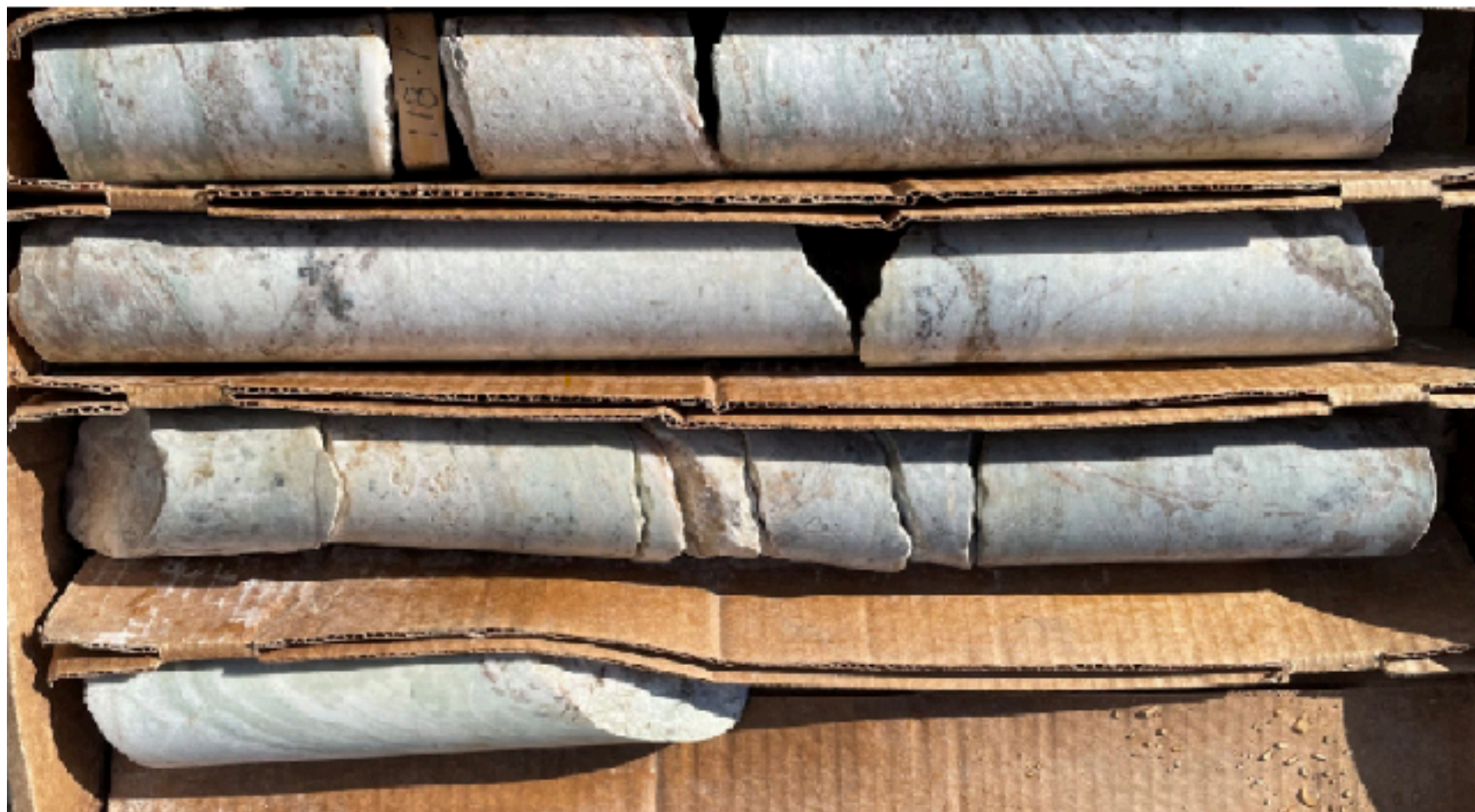
Localized bornite mineralization in calc-silicates @ 120' in BM22-02
