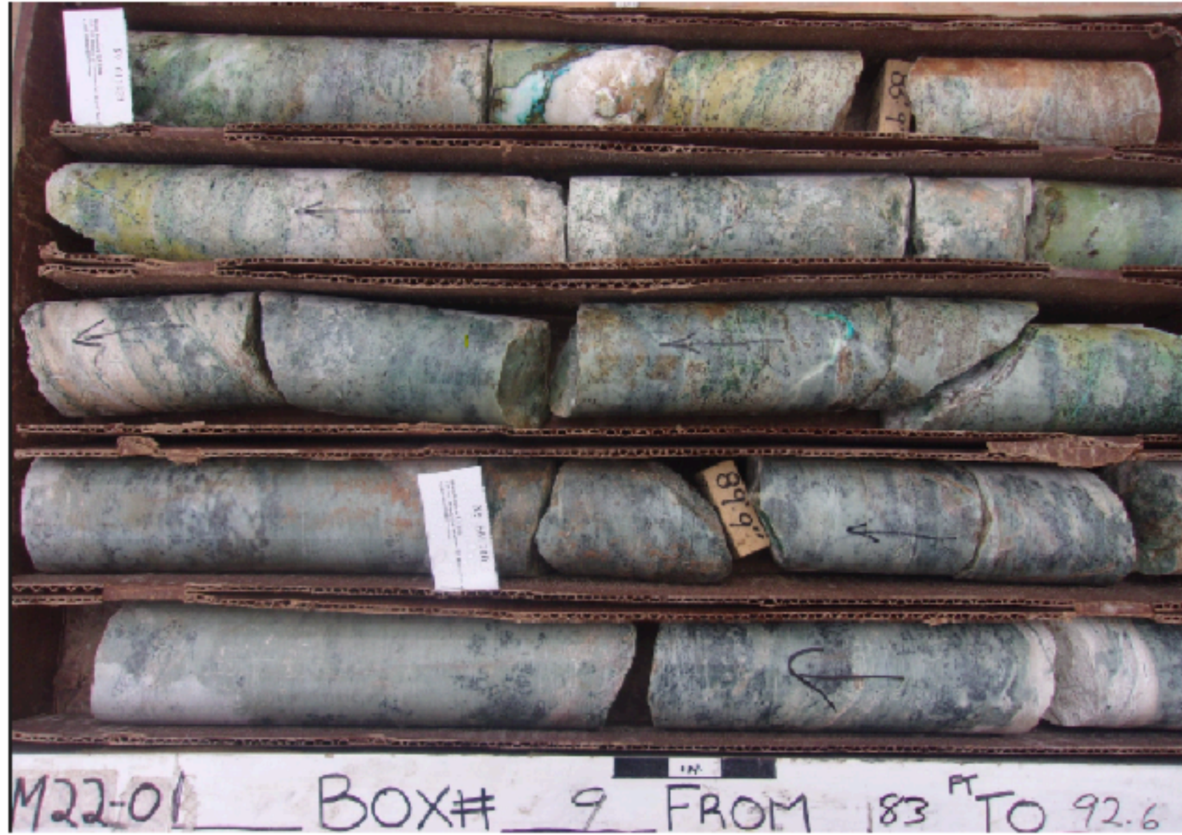
Strong bornite + Copper oxide in BM22-01 (83' - 92.6')
