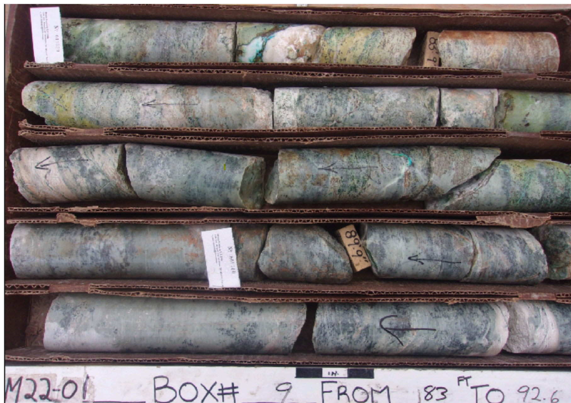
Strong bornite + Copper oxide in BM22-01 (83’ - 92.6’)
