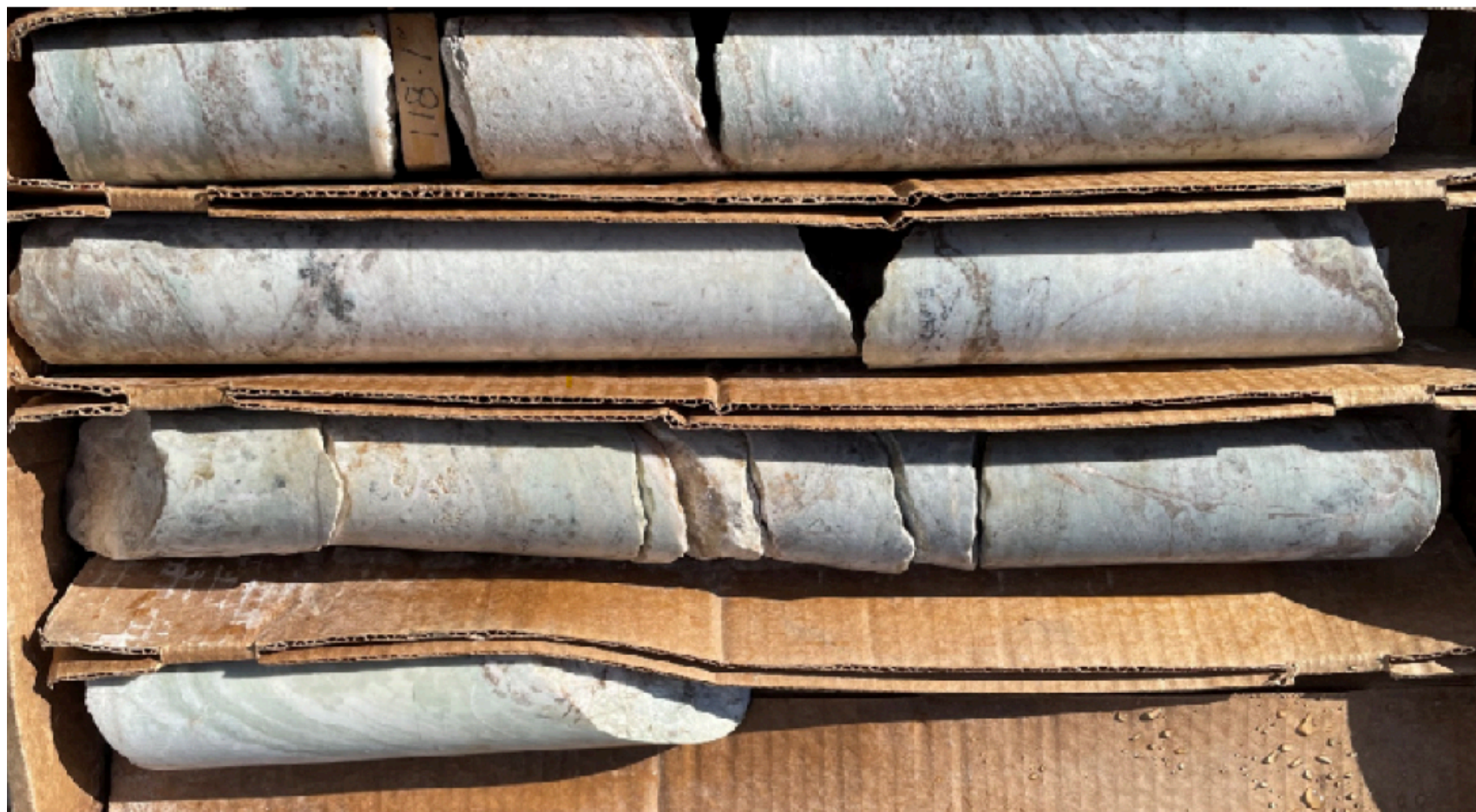
Localized bornite mineralization in calc-silicates @ 120' in BM22-02
