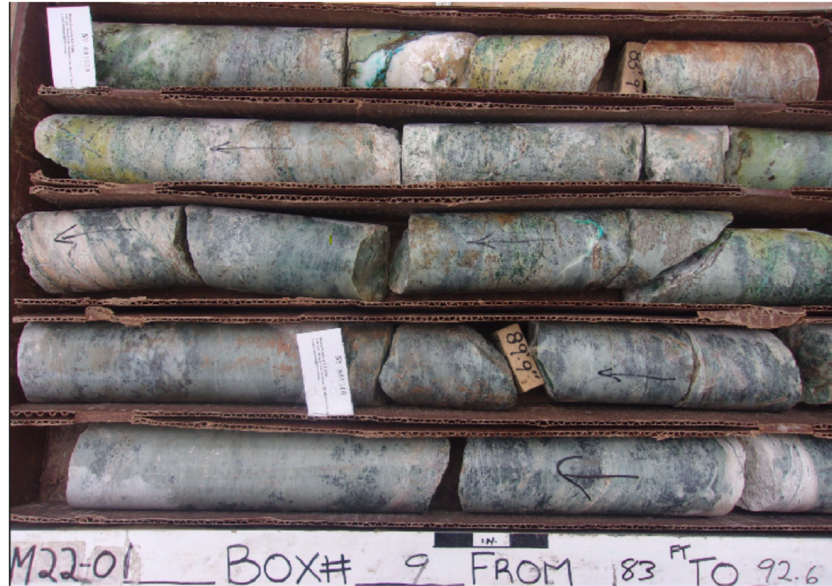
Strong bornite + Copper oxide in BM22-01 (83' - 92.6')
