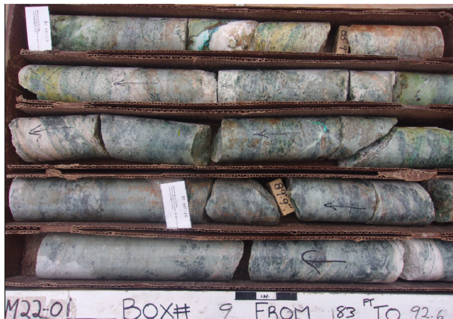
Strong bornite + Copper oxide in BM22-01 (83' - 92.6')
