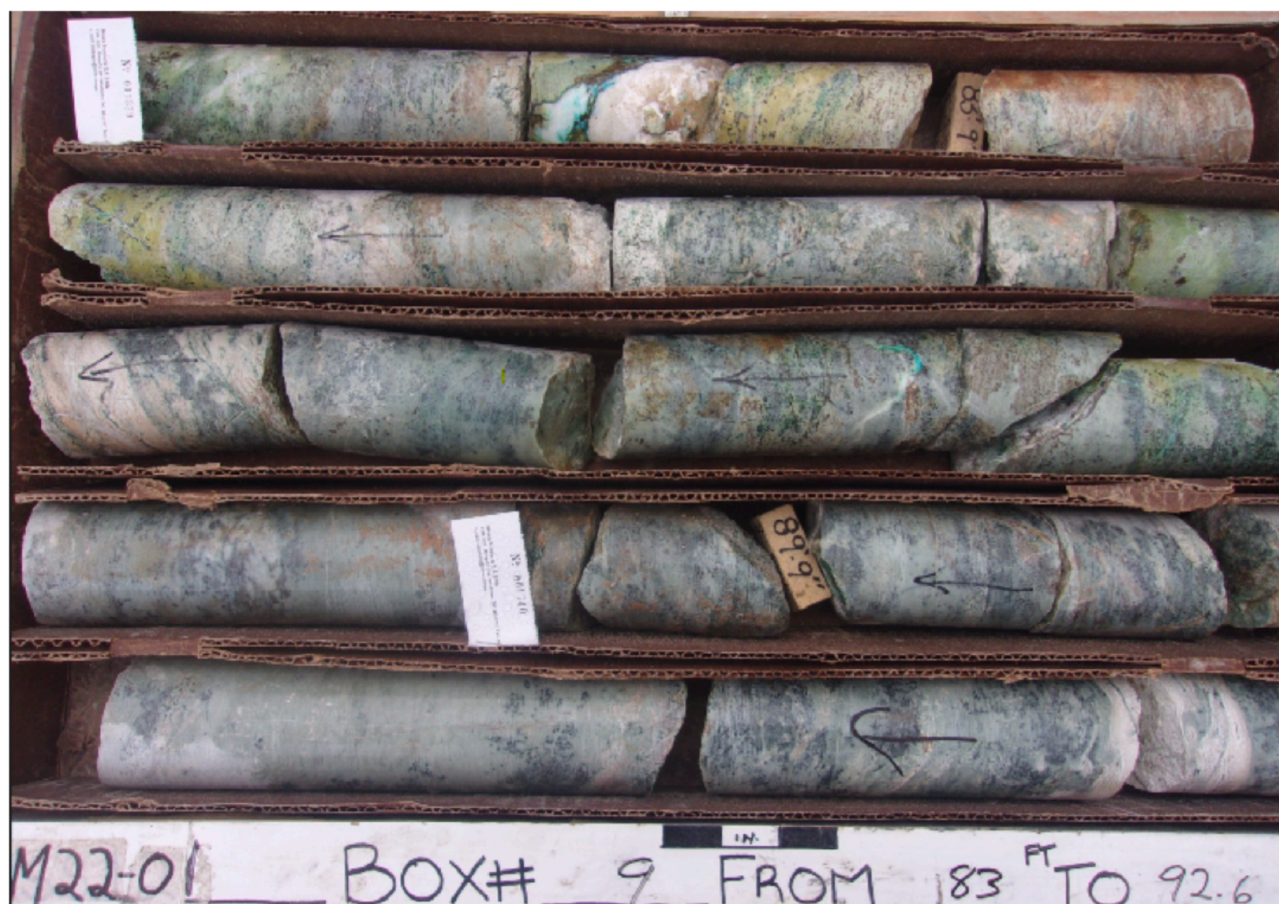
Strong bornite + Copper oxide in BM22-01 (83’ - 92.6’)
