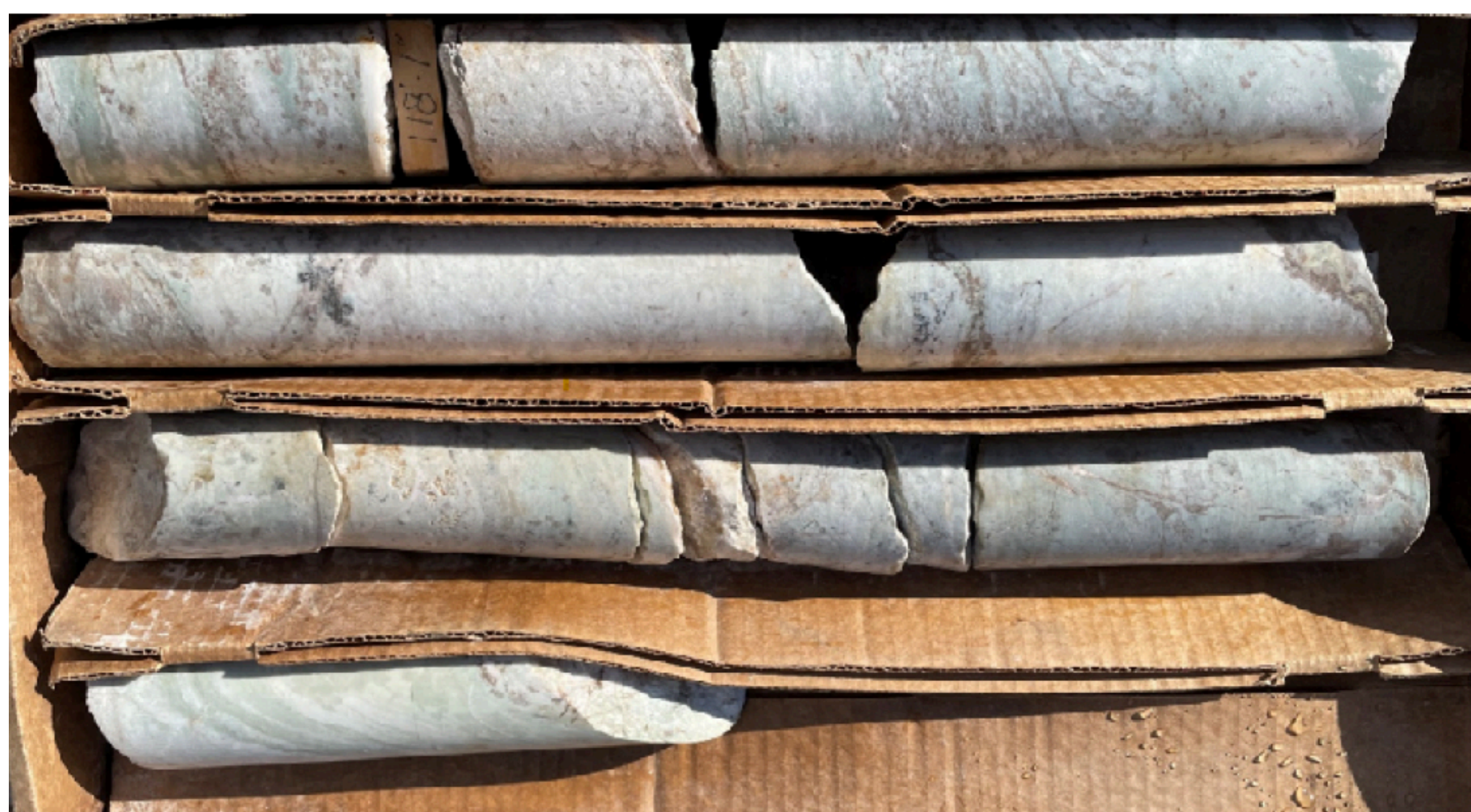
Localized bornite mineralization in calc-silicates @ 120’ in BM22-02
