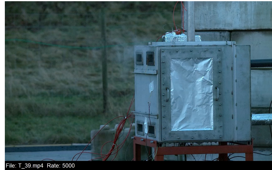
Test 39 - LH2 ignited release in cold box (video courtesy of HSE)
