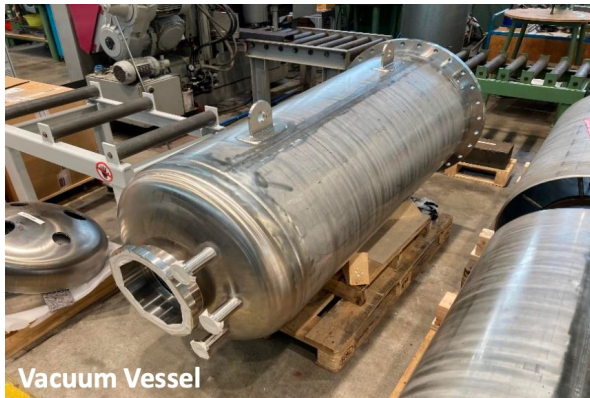
LH 2 tank (images courtesy of KIT)
