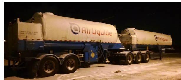
Example of A-Double train configuration operated in Canada (LN 2 )
