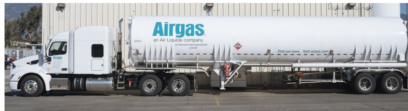
Example of Airgas LH 2 Jumbo trailer manufactured by Worthington
