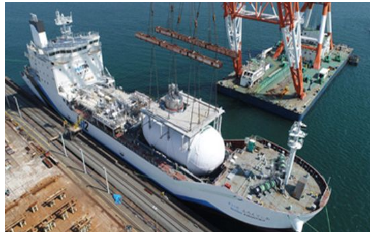
The world's first LH 2 carrier ship SUIISO FRONTIER launched in December 2019 in Kobe, Japan (HySTRA project)
