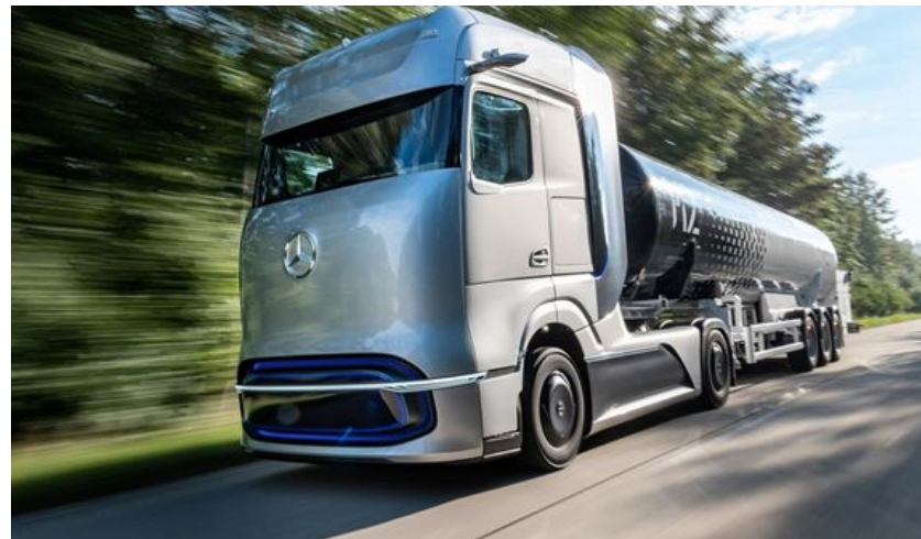
Mercedes FC truck GenH2 concept with LH 2 storage
