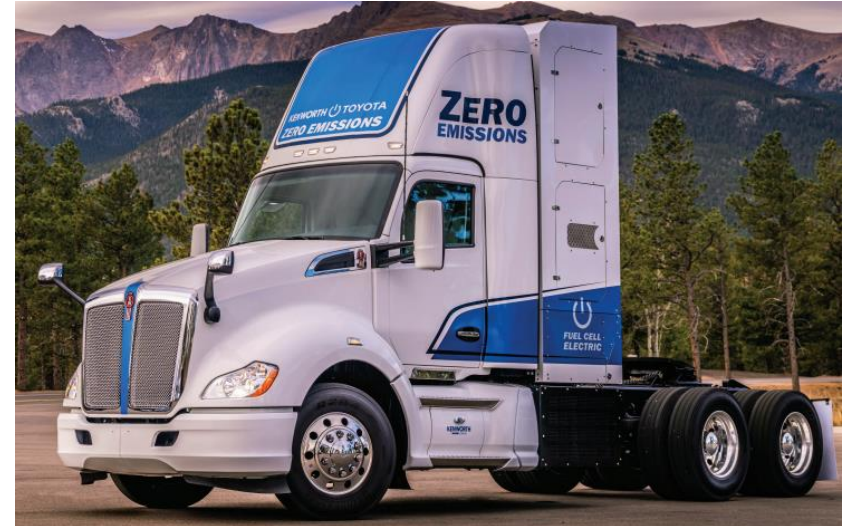
Back-of-cab 700 bar storage system
