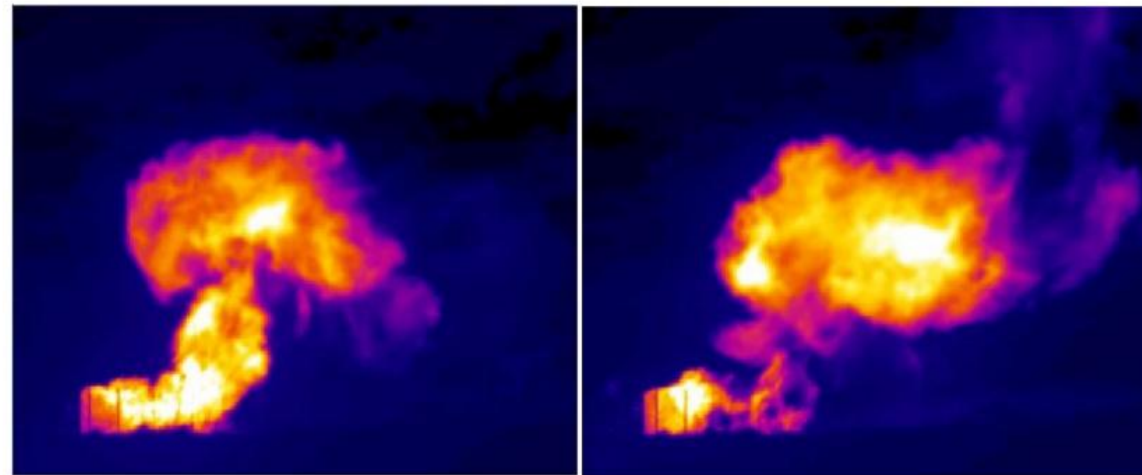
Comparison between fireball caused by (a) the initial flash fire and (b) the secondary explosion.
