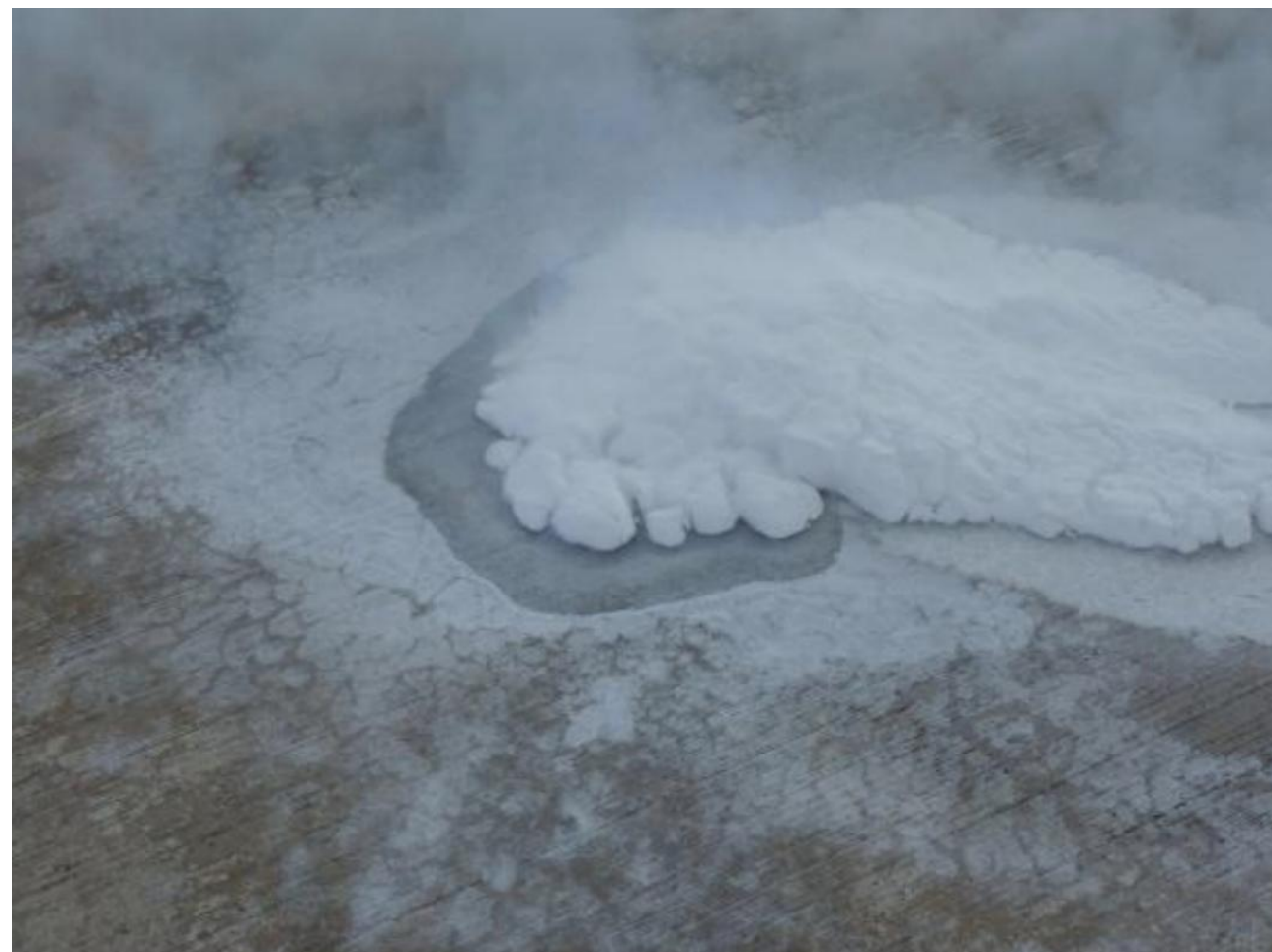
Condensed air following liquid hydrogen release
