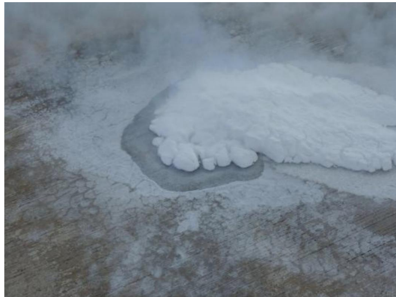
Condensed air following liquid hydrogen release
