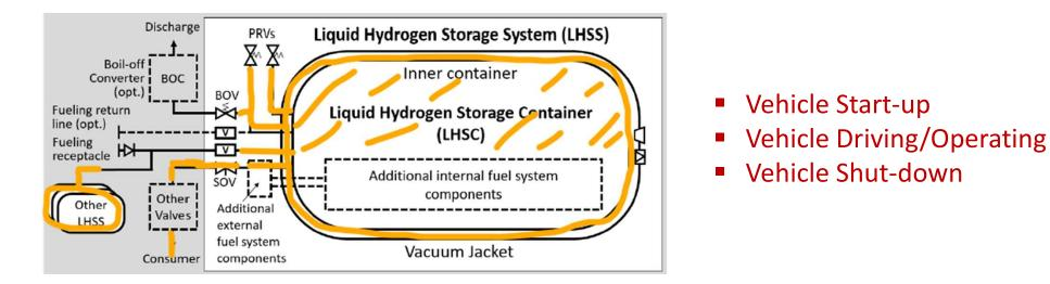
This three phases and related nodes correspond to the ramp-up, operation and ramp-down of the power train using hydrogen supplied by the storage
