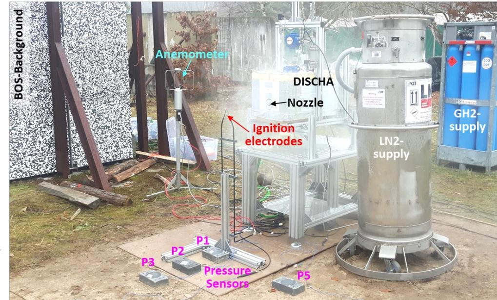
Tests at **ambient temperature** and **approx. 80 K**
