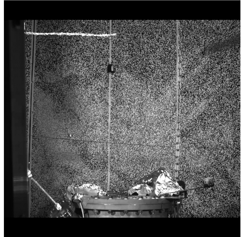
DALSA: Test of 06.08.2026; vacuumized 10e-2 ; rupture pressure 13,2bar; NO heater used. IGNITED
