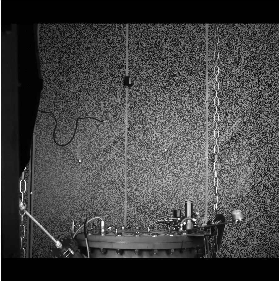
DALSA: Test of 31.07.2026; vacuumized 10e-2 ; rupture pressure 14,1bar; NO heater used. UNIGNITED
