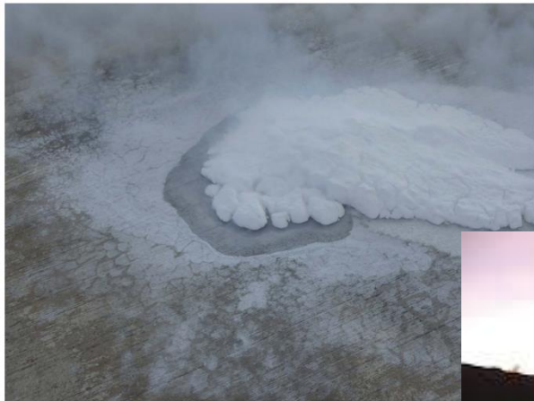
Experimental release of LH2 previously performed at HSE (Hooker et al., 2012)
