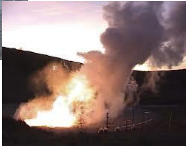
Experimental release of LH2 previously performed at HSE (Hooker et al., 2012)
