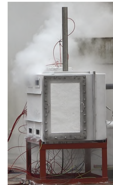
after valve closed (915 s), showing residual vapour from upper passive vent.
