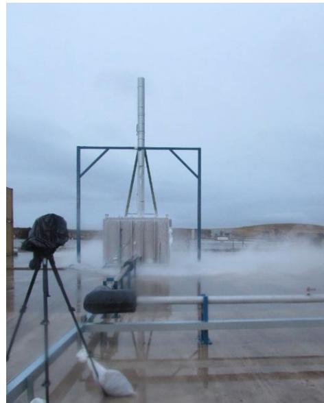
LH2 indoor release tests previously performed by DNV (Aaneby et al., 2021)
