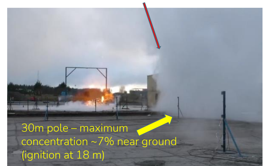
NPRA LH2 test 5 – 2 nd release ignition 18 m successful – flame propagation stops >8%
