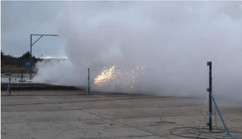
NPRA LH2 test 5 – 1 st release – ignition at 24 m and 18 m failed
