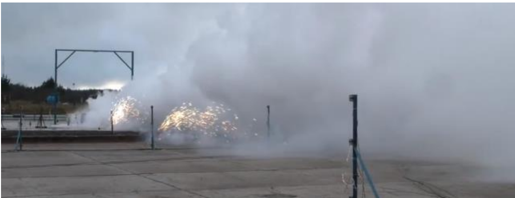
NPRA LH2 test 5 – 1 st release – ignition at 24 m and 18 m failed
