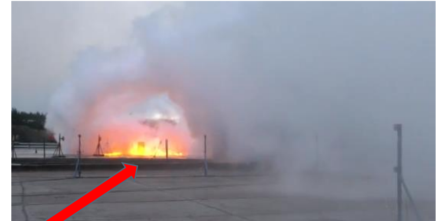
NPRA LH2 test 5 – 2 nd release ignition 18 m successful – flame propagation stops >8%
