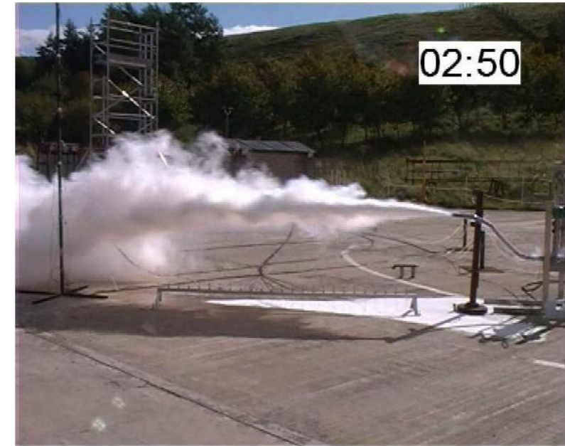
Test 7: Horizontal release from a height of 0.86 m [2]
