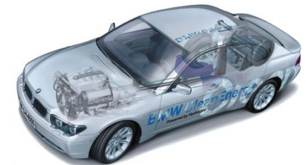
A 7 Series BMW with hydrogen IC engine and LH 2 storage
