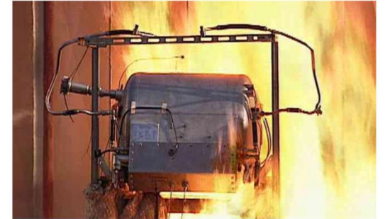
Figure 11: Bonfire test of a liquid hydrogen fuel tank (Source: BAM)
