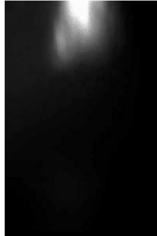
Ignition kernel forms but does not form jet flame
