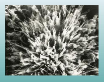
Situation after 29 days. Pores are blocked because of the crystals.
