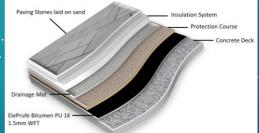
Under green roofs a root barrier and drainage system is required. Typically it is covered by a protection layer to prevent damage to the coating.
