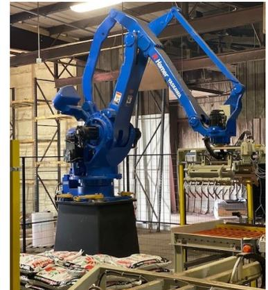
This robot is 13 feet tall 3,800#, and can stack a pallet in under 2 minutes
