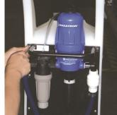
B. Install pickup hose into DosaCart lid (bottom-up).
