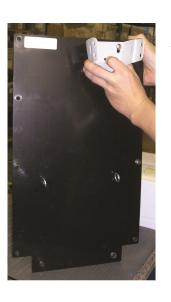
B. Remove plate and attach the Dosatron unit bracket for your unit (see note below) on the same side as the eyebolts,
