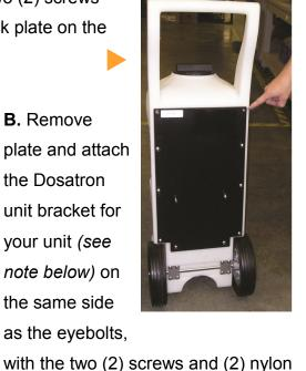
**NOTE**: Use the D14 or D116 unit bracket, two (2) screws and (2) nylon locking nuts provided in the hardware bag.
