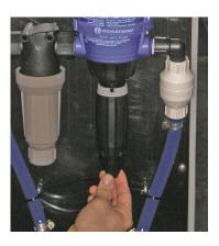
**D.** Place hose nut onto hose, insert pickup hose onto bottom end of unit barb.
