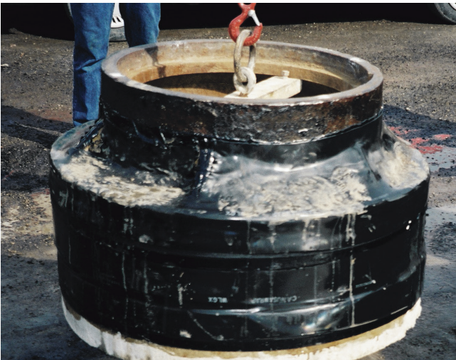
WrapidSeal™ adhesive strength demonstrated with vertical lift.
