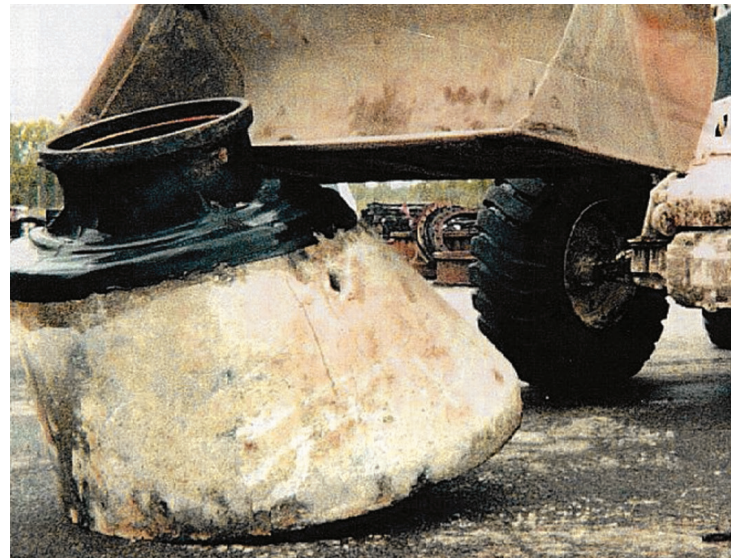
Impact force depicts shear resistance of WrapidSeal™
