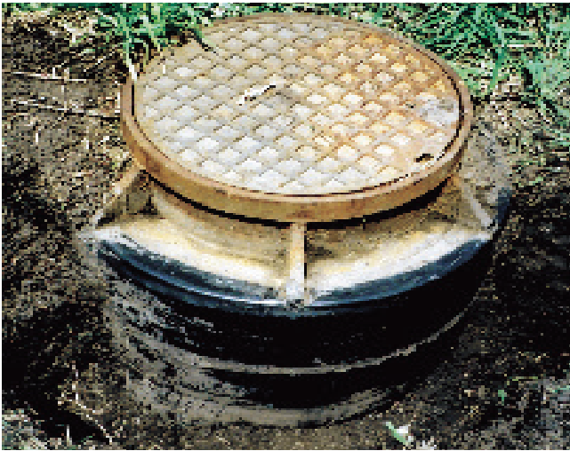
Excellent soil stress resistance after 7 freeze-thaw cycles.
