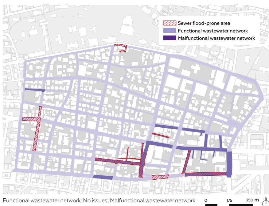
Figure 40 Street mapping of wastewater network
