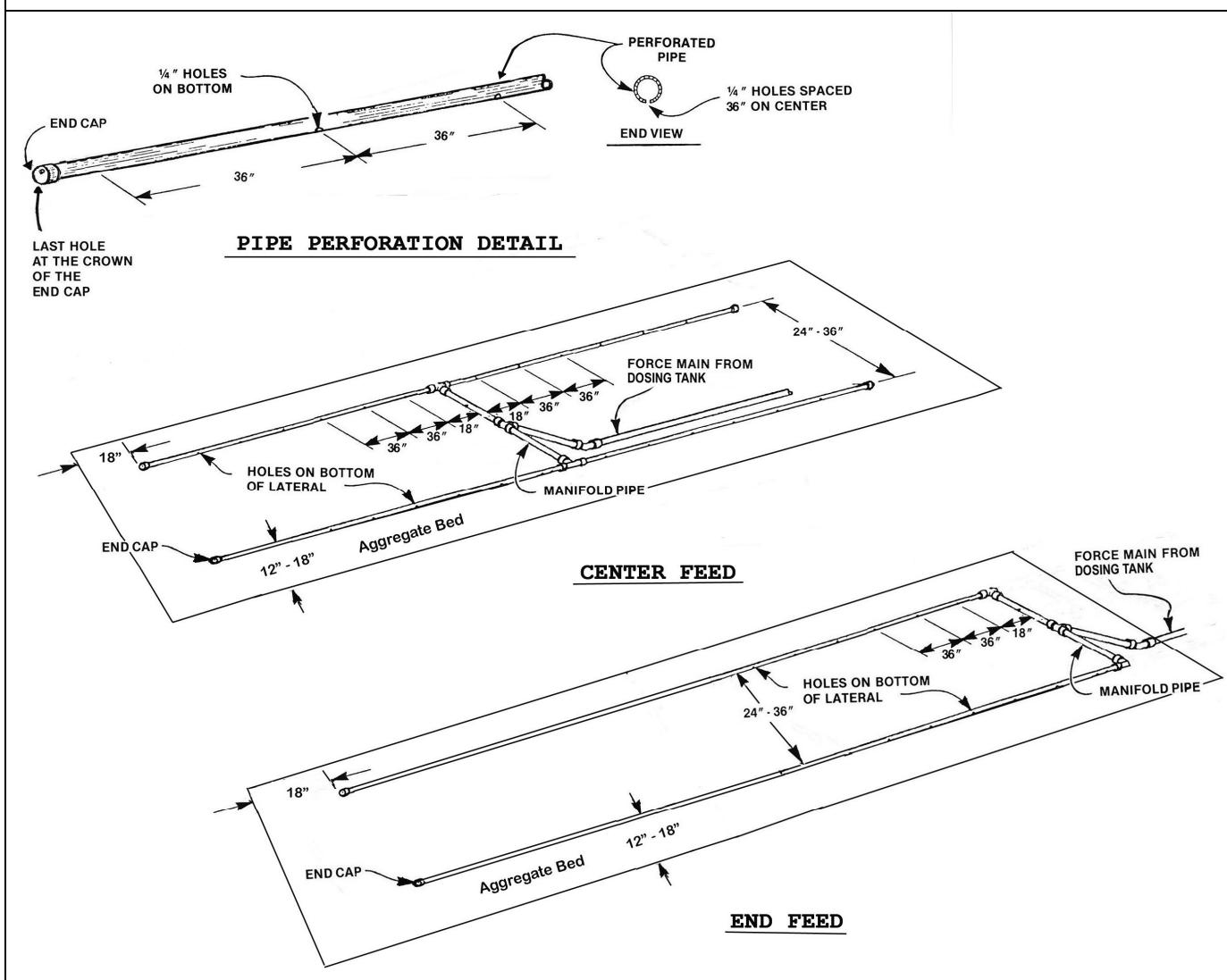
(3) Pressure distribution laterals shall be attached to the manifold using nondirectional fittings designed to withstand the required pressures exerted on them.
