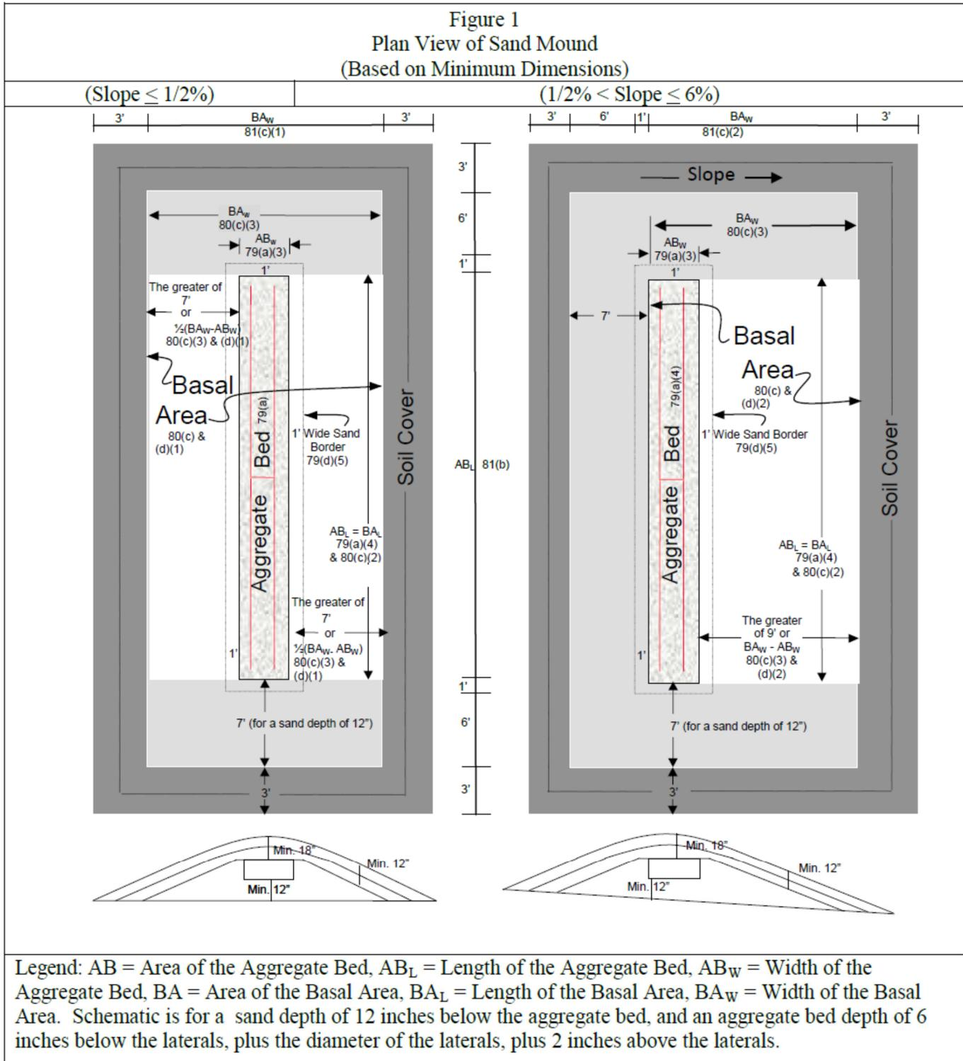
**410 IAC 6-8.3-80 Elevated sand mound on-site sewage systems: design of basal area**
