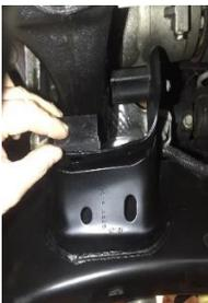
Once the space between the bottom of the motor mount and the motor mount frame bracket is sufficient to accommodate the bump stop, the bump stops can be positioned and installed,
