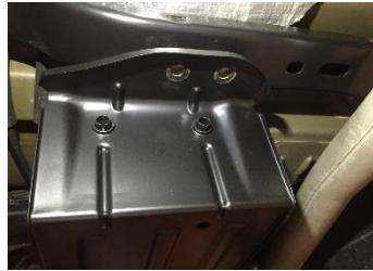
7b. On four door models the upper frame cross member located behind and above the transfer case does not have the two factory bolts like the two door models do, therefore two holes must be marked out and drilled by using the factory located hole in the upper frame cross member as a starting point for measurements.
