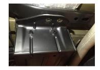
7b. On four door models the upper frame cross member located behind and above the transfer case does not have the two factory bolts like the two door models do, therefore two holes must be marked out and drilled by using the factory located hole in the upper frame cross member as a starting point for measurements.
