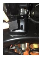
D. Start on the left side motor mount and position the polyurethane bump stop in the space between the bottom of the motor mount and the motor mount frame bracket. If the space between the bottom of the motor mount and the motor mount frame bracket is smaller than the bump stop, then try one of the two options. Note the bump stop must fit tightly between the bottom of the motor mount and the motor mount frame bracket.
