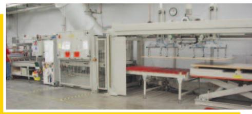
Switching the manufacturing process from a cold press to a Joos throughfeed hot press and stacking line has saved A-dec considerable production time and increased profits.
