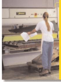
To improve its efficiency and quality in the pressing area, Craftwood replaced its older oil-heated hot presses with water-heated ones from Joos USA. The 4-foot by 8-foot stationary press, pictured left, was purchased by Craftwood in October 2001. Craftwood Industries supplies many of the top office furniture companies with veneered OEM components, which it produces using two Joos water-heated veneer presses.
