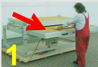
1 Withdraw table and place the sheets or plastics board in position.
